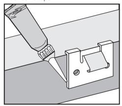
■ In addition, coat the edges of the spring clips with silicone sealant.
